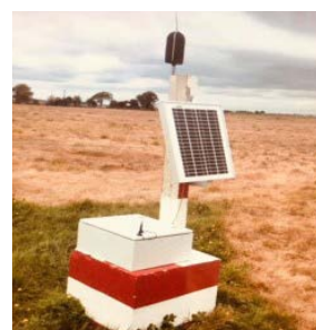
Acoustic meter powered by 100% renewable energy.
