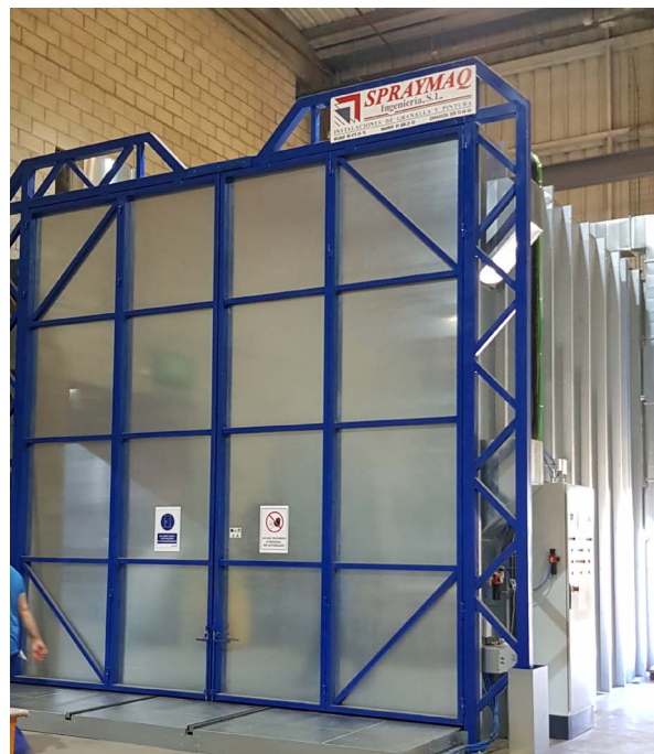
Megaplas. Installed projection booth.
