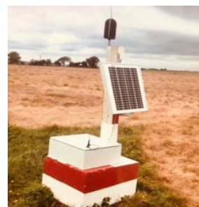
Acoustic meter powered by 100% renewable energy.
