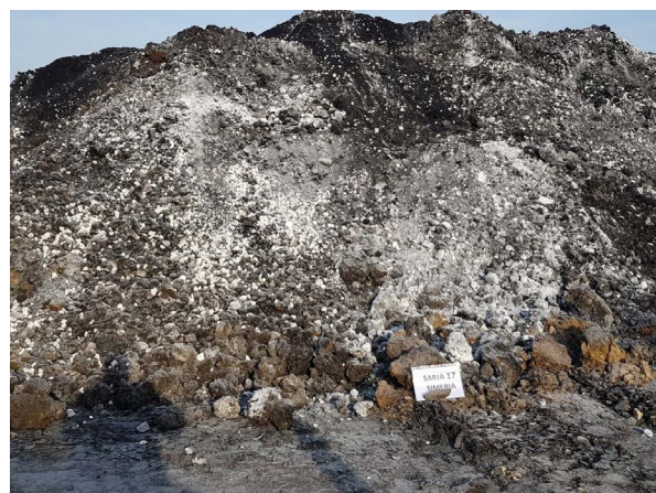
Bioremediation process carried out on contaminated soil collected from the railway line between Gurasada and Simeria. The micro-organisms that develop in the soil through the bioremediation process break down the hydrocarbons and release carbon in the form of CO 2 into the atmosphere as matter, and an inert or humic material that can be reused on the construction site.
