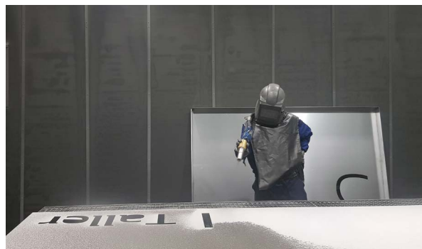
Megaplas. Shot blasting by a worker with the corresponding PPE.
