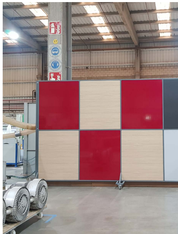
Sound-absorbing panels installed to attenuate noise emissions in the areas surrounding the milling machine.
