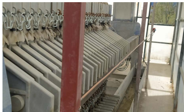
Inside the press filter. The sludge cloud remaining in a concentrated suspension state achieves accelerated flocculation. Water filtered through the sludge bed is collected completely free of solids.
