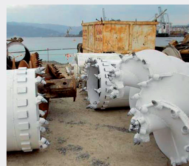
Special tools with widia teeth for rotation drilling of the pile-driving in rock.
