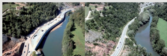
Aerial photograph of the River Ter before and after the construction of Wall 13.5.
