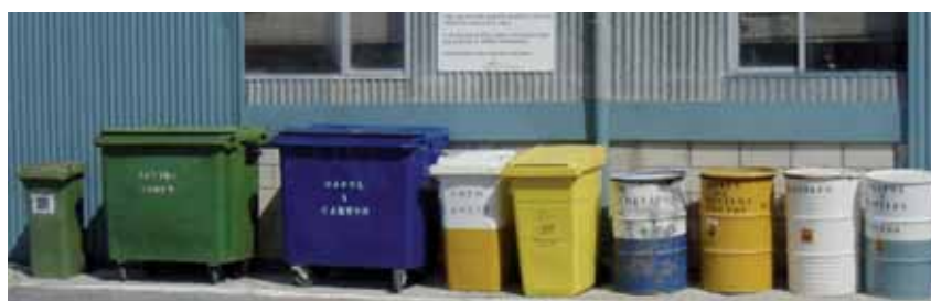
It is necessary to reserve a special place to separate and store the great diversity of packages that concentrate on the site. Its management involves delivery, either to the stored system and return or an integrated management system if they are submitted to some of these or to a financial agent for recovery, recycling or power production.
