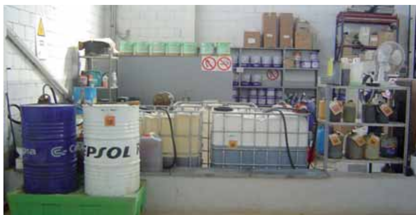
It is very important to provide correctly cordoned-off and signposted areas for temporarily storing dangerous wastes that must remain closed when not in use. This prevents spillages, tipping and mixtures of dangerous wastes.
