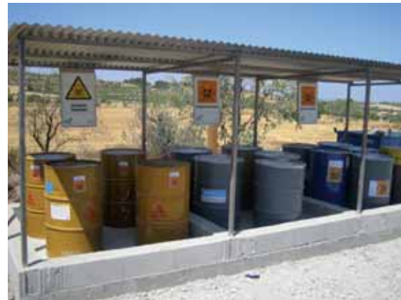
The RPs are deposited in tubs that are suitably impermeable, separated and labelled.
