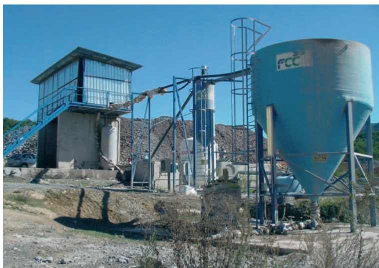
In projects that produce important quantities of waste, such as tunnels, more sophisticated cleaning devices are sometimes installed for neutralising pH, decanting, sludge drying, etc, to meet quality requirements that are above those required
