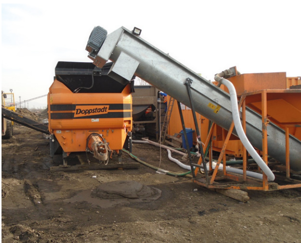
With the Doppstadt SM 620 Trommel Screening Machine a closed circuit is generated to decontaminate the ballast, allowing the water used to be reused and waste to be properly disposed of.
