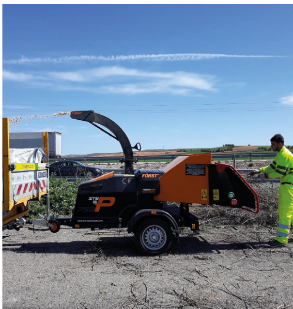
Bio shredder to reduce the size of branches.
