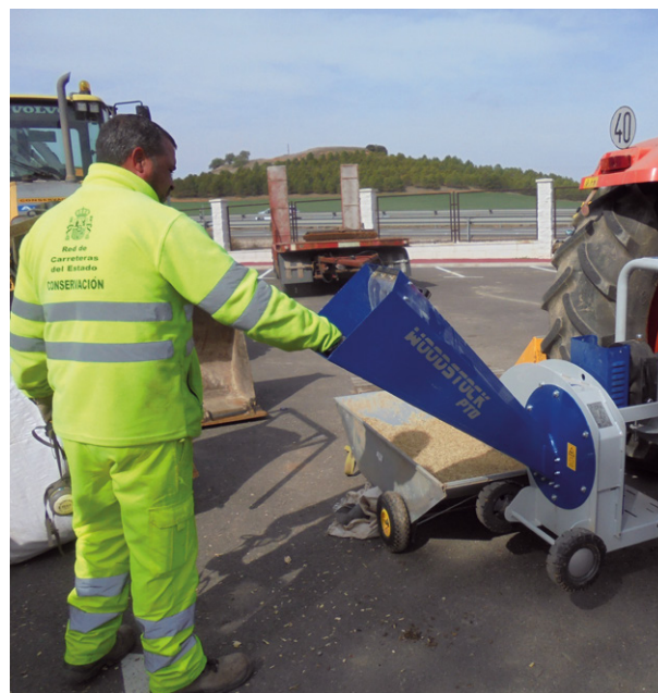
Second phase of crushing to produce sawdust.
