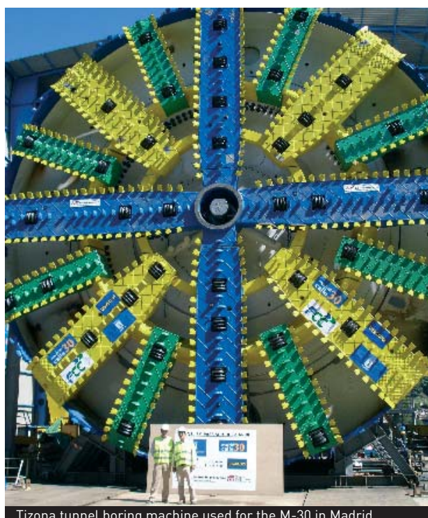
Tizona tunnel boring machine used for the M-30 in Madrid
